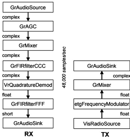
Figure 3. NCSA GNU Radio FM transceiver block diagram.
