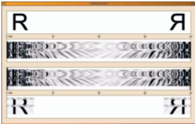
Figure 9. Illustration of overmodulation.
