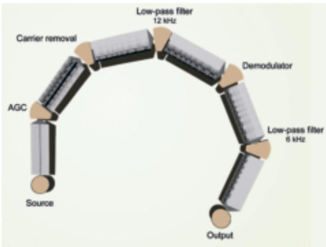
Figure 11. NCSA GNU Radio FM receiver in 3D.
