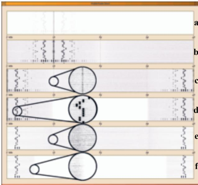
Figure 5. Signal processing stages in the FM receiver, with details of a sound-card artifact (c), DFT leakage (d), noise reintroduced by modulation (e), and low-pass filter cutoff (d).
