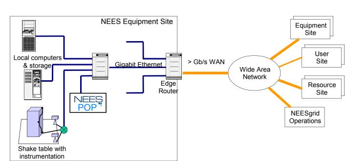
NEESgrid is an integrated network that will link earthquake engineering research sites across the country, provide data storage facilities and repositories, and offer remote access to the latest research tools. The NCSA Grid Technologies group is responsible for Grid software deployment for the NEESgrid project.
